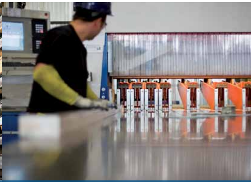
3 Plates are cut accurately to size on CNC plate saws
