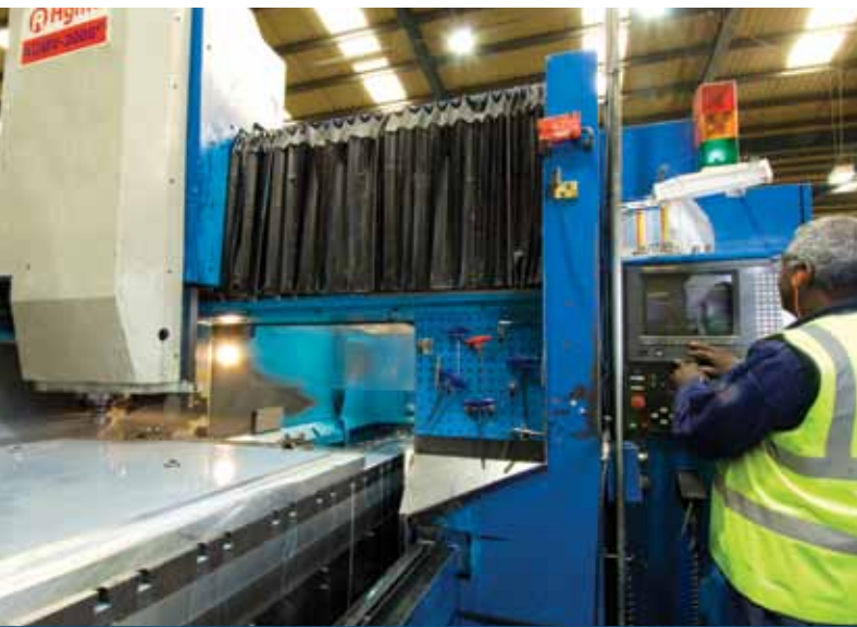
4 Nested billets are machined and tooling holes drilled
